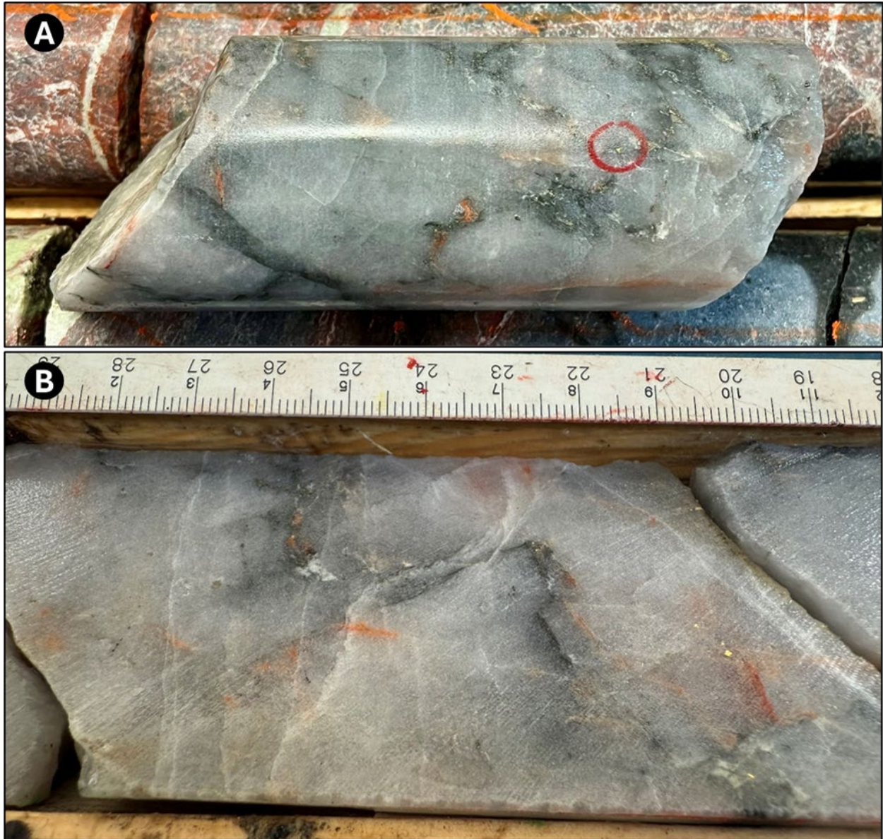
Figure 1 - Core photo of SD-25-559 showing VG. Core is NQ size core with a diameter of 47.6 mm, B is a crosscut of the core.
