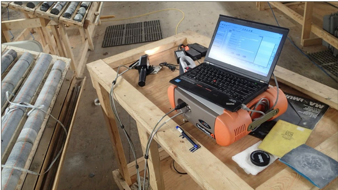
Figure 10-5: TerraSpec 4 Hi-Res Mineral Spectrometer and Data Acquisition Computer on the Rolling Table Used to Acquire SWIR Data on Historical Core
