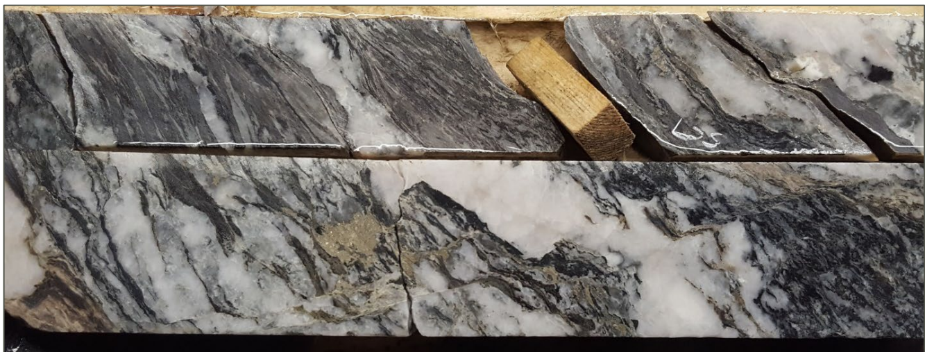
Figure 7-17: Quartz-Tourmaline Veins of the Minto Deformation Period in the Surluga Deposit
