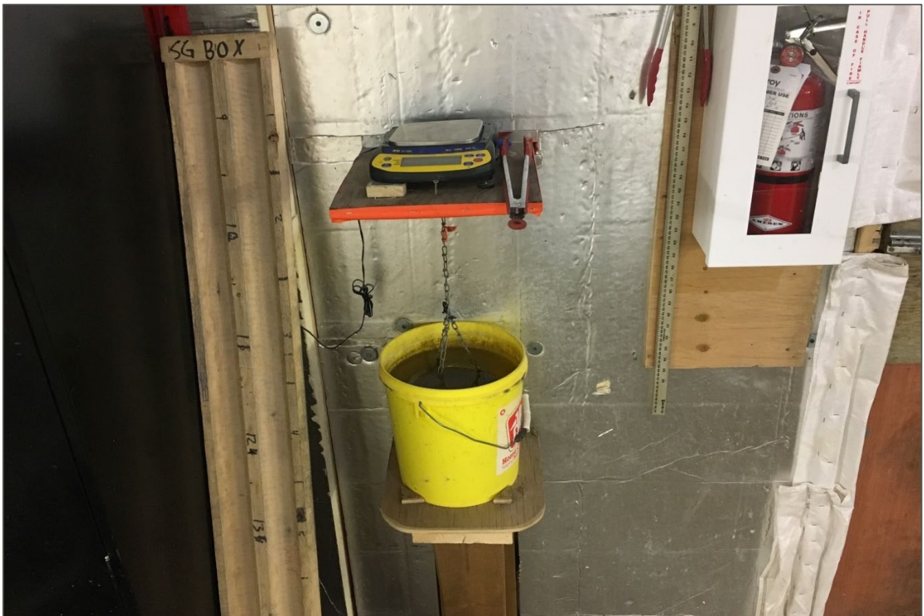
Figure 11-3: SG Measurement at Red Pine's Core Logging Facility
