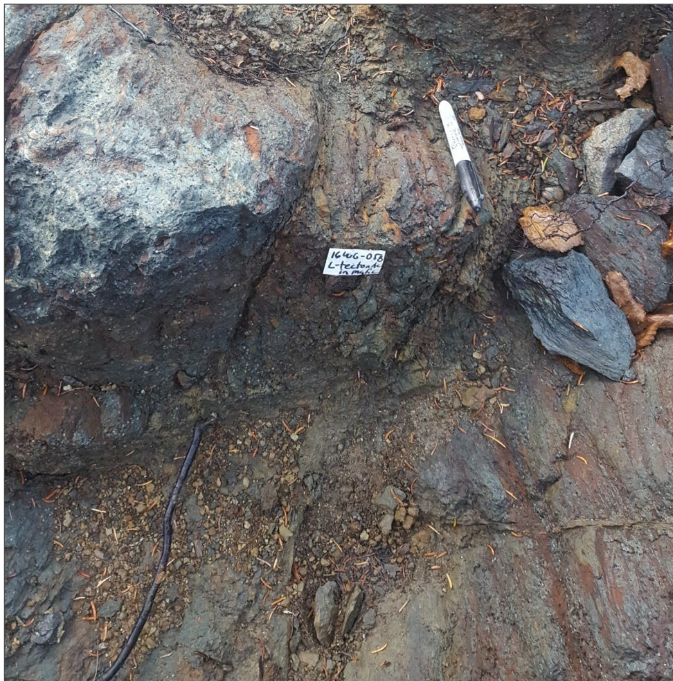
Figure 7-12: Characteristic Stretching Lineation of the Wawa Gold Corridor Preferentially Partitioned in a Mafic Dyke (William Gold Zone)
