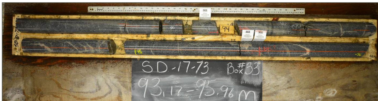
Figure 7-22: Sericitic Alteration Fronts Formed in the Shoulders of the Wawa Gold Shear Zone
