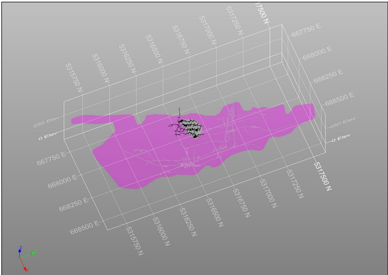
Figure 14-11: Block Model Volume Excluded from Mineral Resource to Account for Historical Mining
