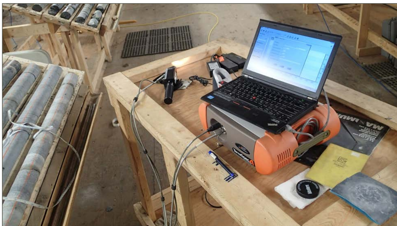
Figure 10-3: TerraSpec 4 Hi-Res Mineral Spectrometer and Data Acquisition Computer on the Rolling Table Used to Acquire SWIR Data on Historical Core
