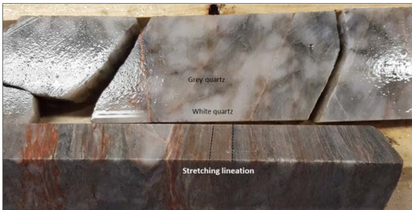
Figure 7-15: Quartz Vein Stretched in the Stretching Lineation Characteristic of the Jubilee Shear Zone
