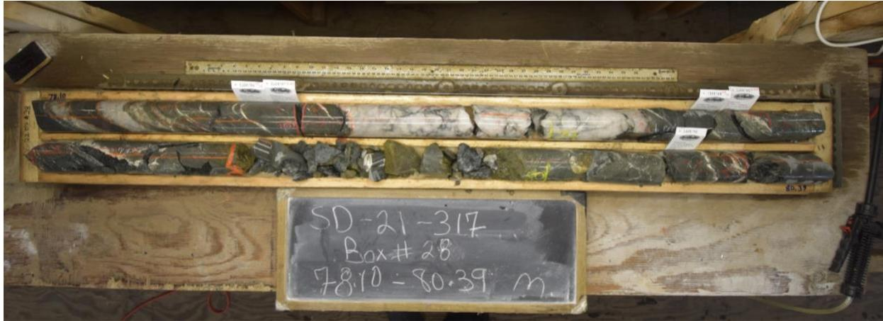
Figure 2 - Quartz veining in the Nyman Shear Zone containing 11.47 g/t gold over 2.73 meters
