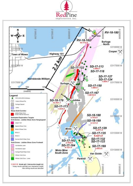
Figure 1 – Plan Map of Drilling Results
